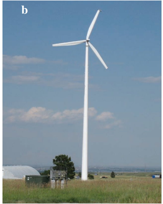
Figure 1. Small wind turbines come in many sizes from micro turbines like the 400 watt turbine above (a) to turbines as large as 50 to 100 kW like the 50 kW turbine pictured above (b).
