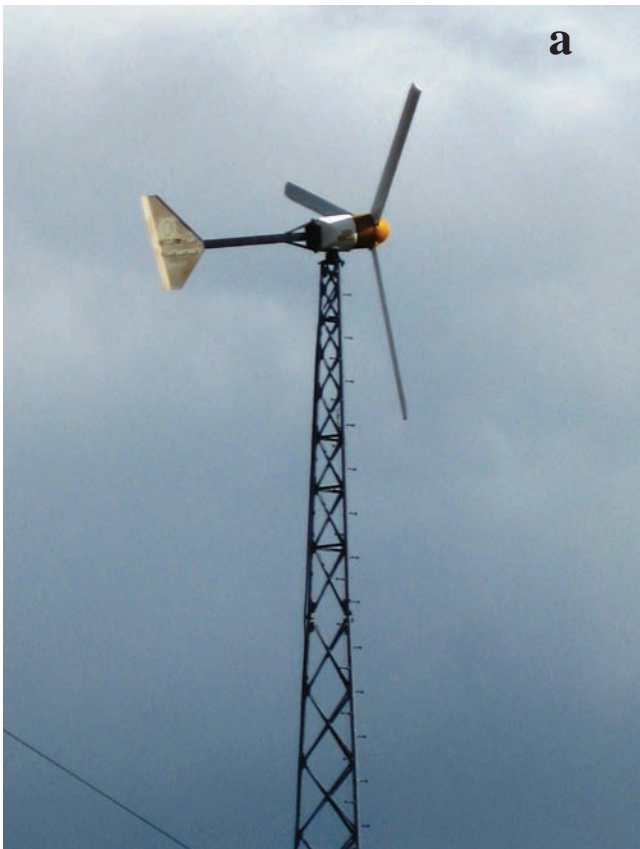
Figure 2. Two common styles of horizontal axis wind turbines are upwind (using tail to face into the wind, Figure 2a ) and downwind (wind blows around tower to reach blades, Figure 2b ).
