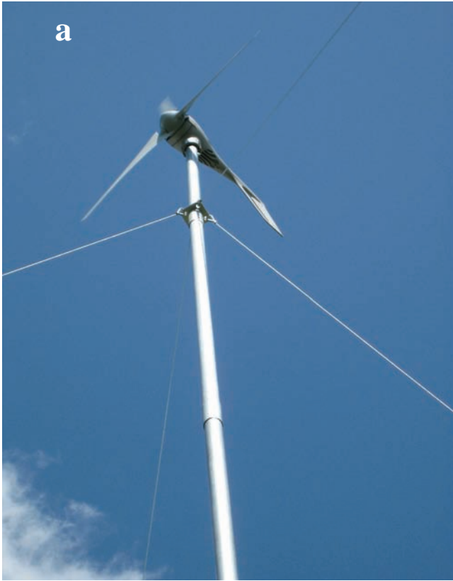
Figure 1. Small wind turbines come in many sizes from micro turbines like the 400 watt turbine above (a) to turbines as large as 50 to 100 kW like the 50 kW turbine pictured above (b).
