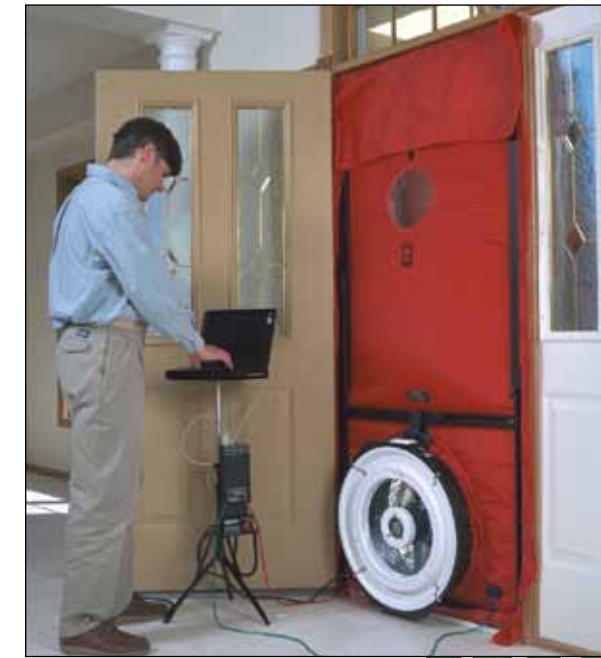
A blower-door test is a key part of a home energy audit.
